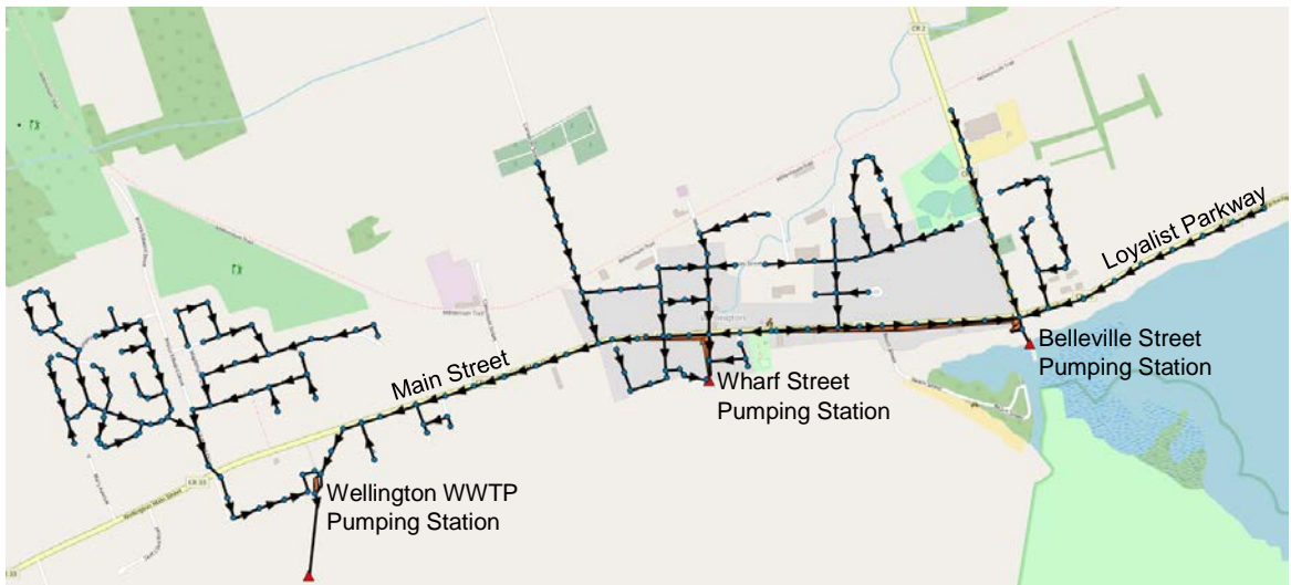
Figure 1.1 – Wellington Sanitary Sewer Plan
