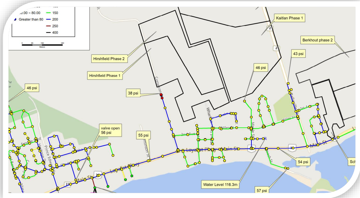
FIGURE 1: EXISTING WATER SYSTEM STATIC PRESSURES UNDER PEAK HOUR CONDITIONS (ADAPTED FROM THIRD-PARTY MODEL)
