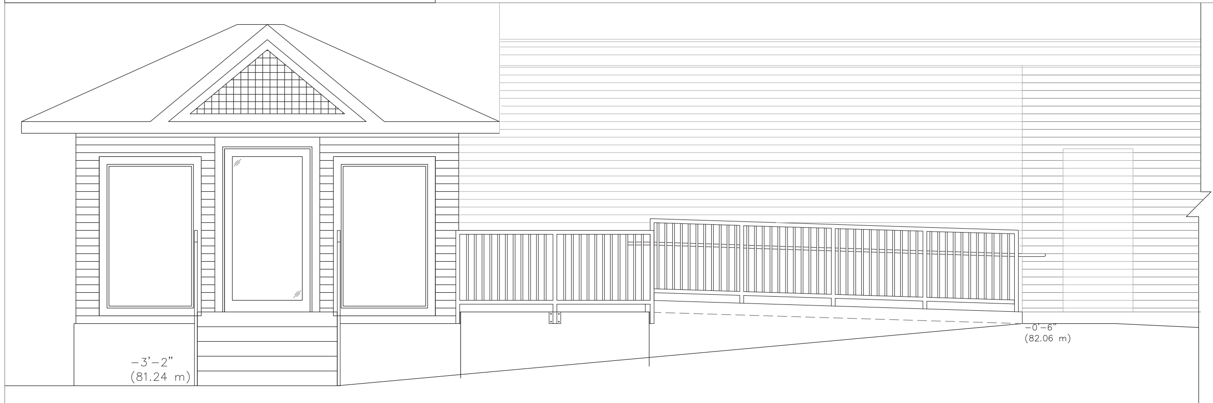
1 STAIR B AND RAMP - ELEVATION A-601C SCALE 1/4" = 1'
