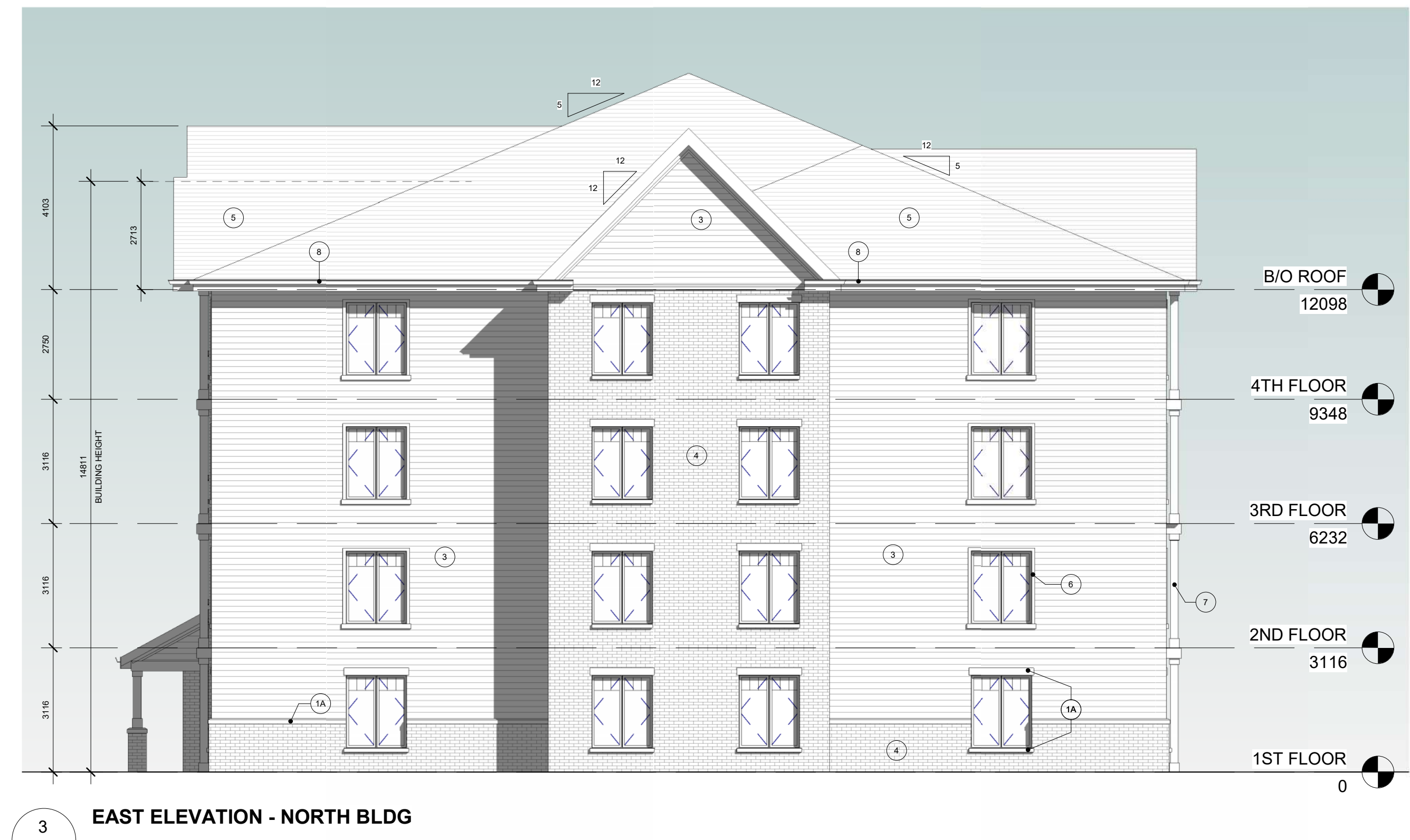
3 EAST ELEVATION - NORTH BLDG A.201 1:100
