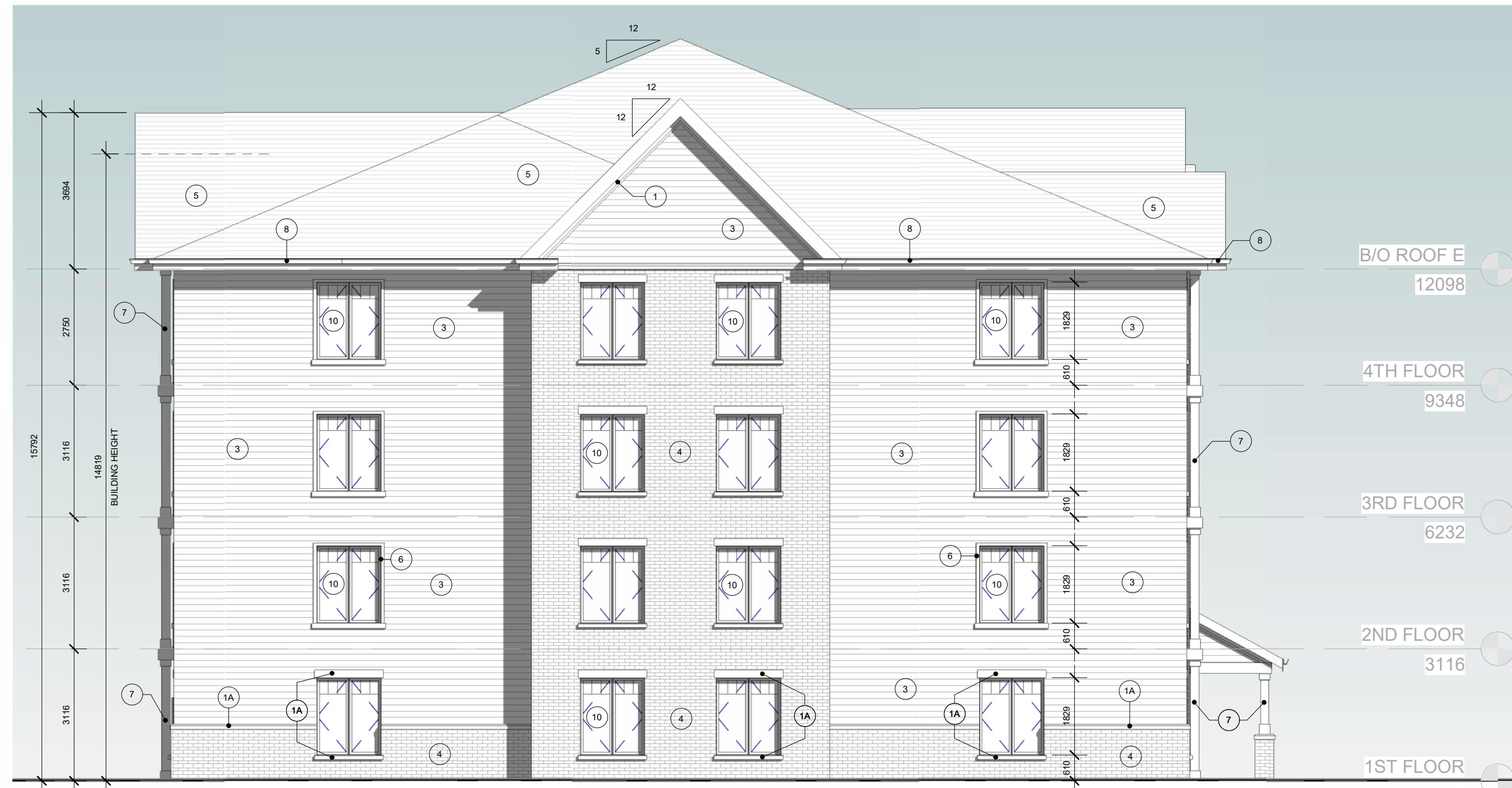
4 NORTH ELEVATION - E BLDG A.201 1:100
