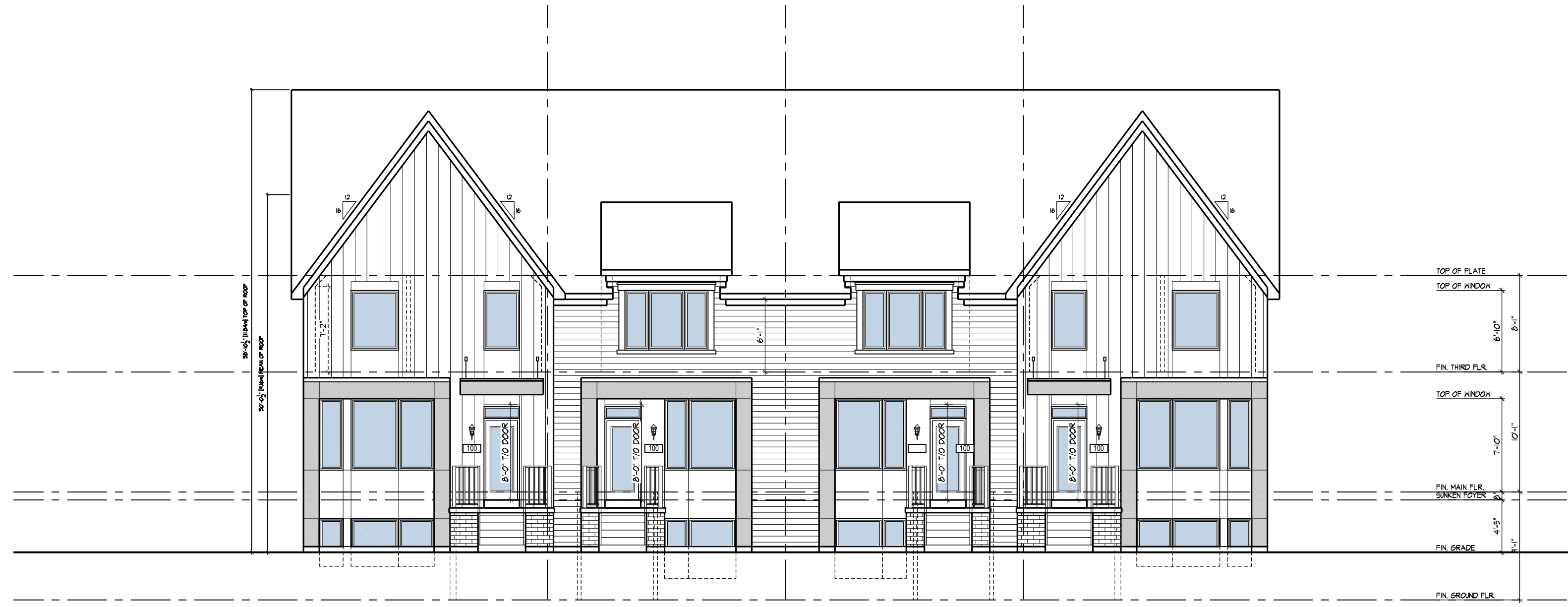
UNIT CDF-03-END UNIT CDF-01 UNIT CDF-01 UNIT CDF-03-END FRONT ELEVATION - CONCEPTUAL DUAL FRONTAGE BLOCK ELEVATION 'A' BLOCK OF 6
