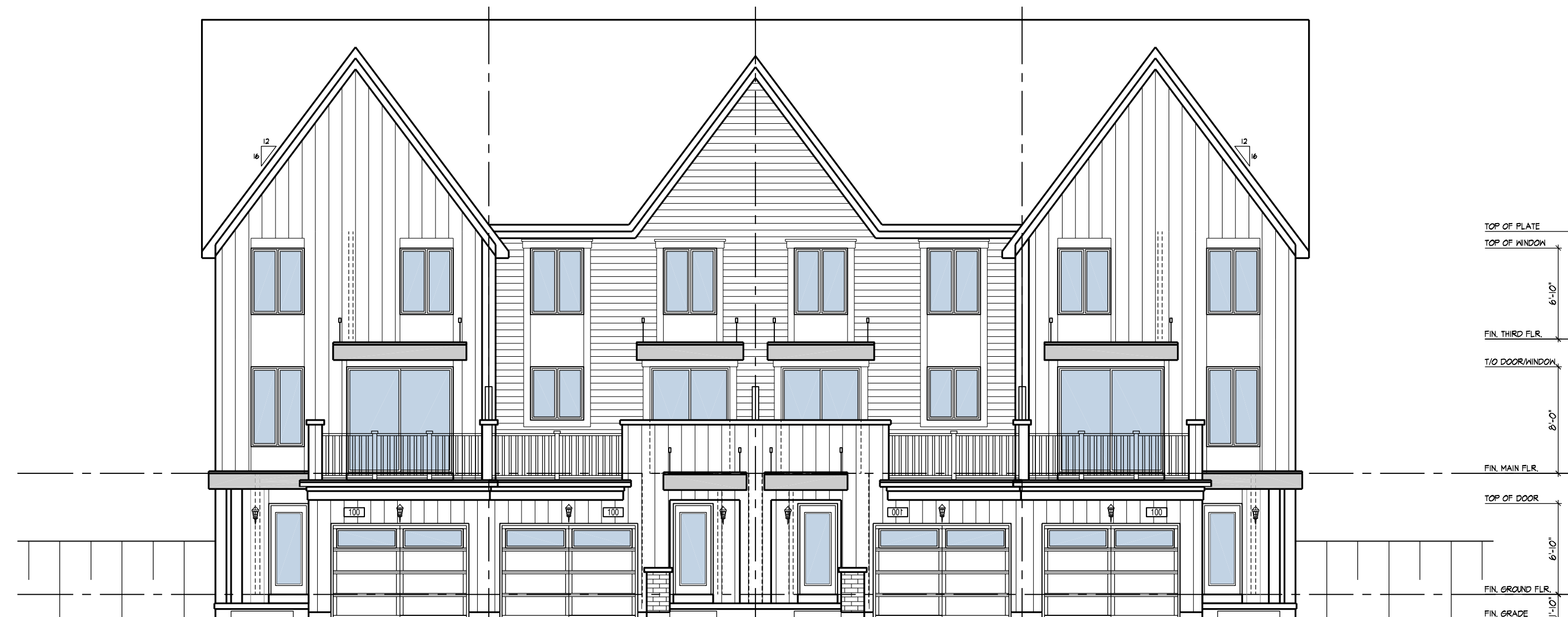
UNIT CDF-03-END UNIT CDF-01 UNIT CDF-01 UNIT CDF-03-END REAR ELEVATION - CONCEPTUAL DUAL FRONTAGE BLOCK ELEVATION 'A' BLOCK OF 6
