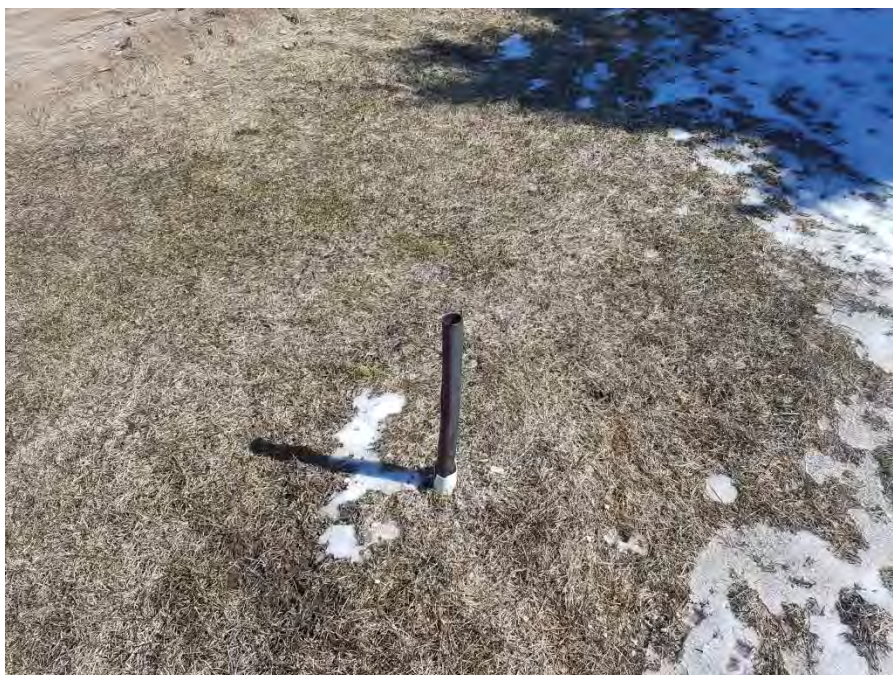
Photo 10 Possible monitoring well on-site
