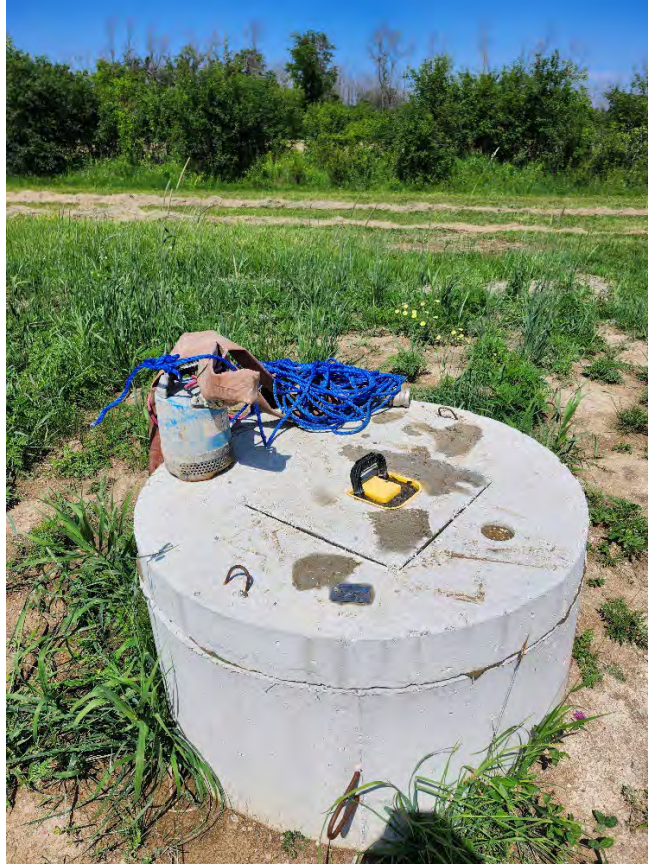
Photo 1: Test well A334420 at proposed severance just prior to the pumping test
