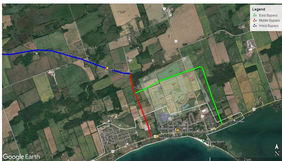
Figure 2-7: Future Collector/Bypass Road – Preliminary Alignment
