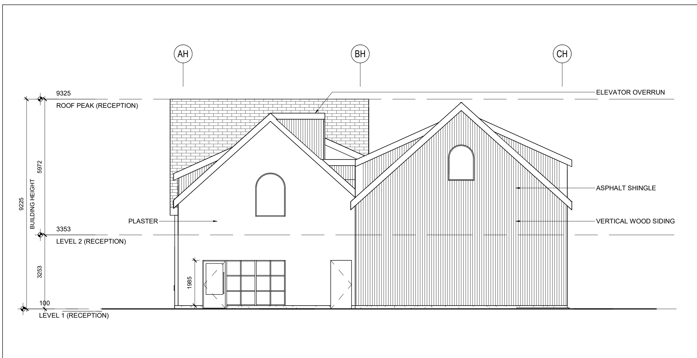
RECEPTION BUILDING - WEST ELEVATION 1 : 100 2 A301b
