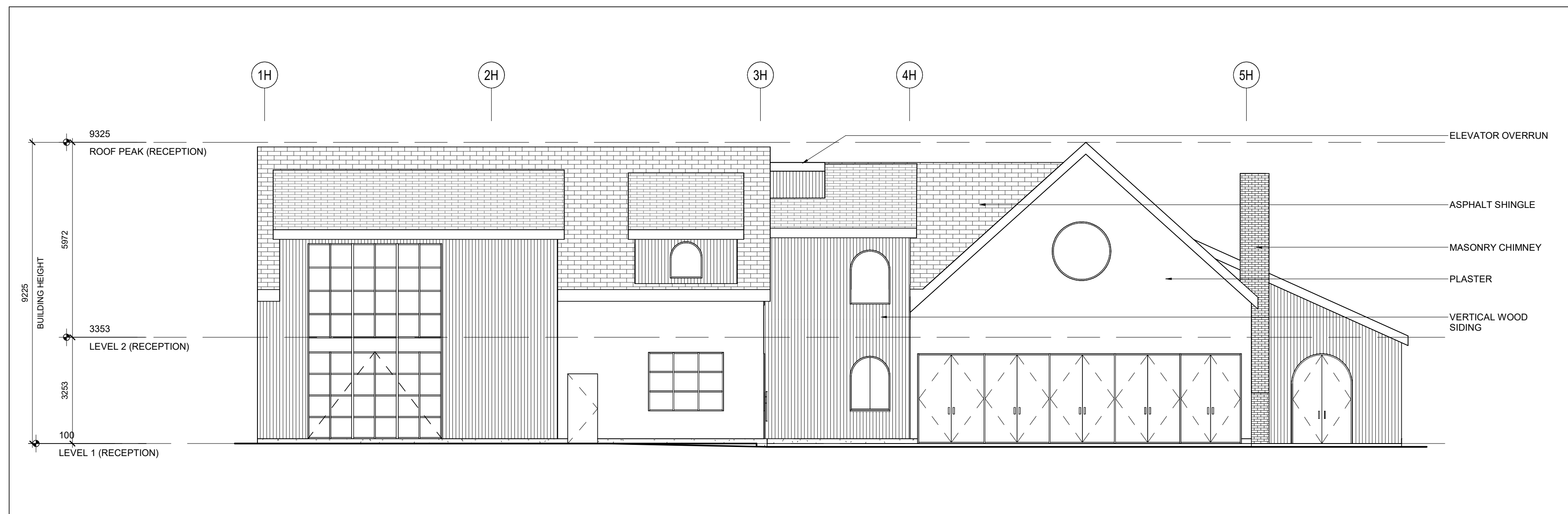
RECEPTION BUILDING - SOUTH ELEVATION 1 : 100 1 A301b
